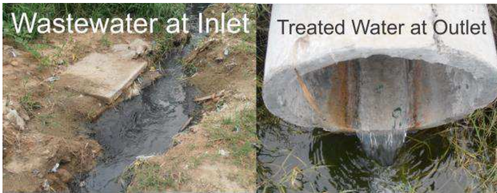
Figure 7. Visual Condition of Water at Inlet & Outlet of Constructed Wetland Project at Village Chattal
